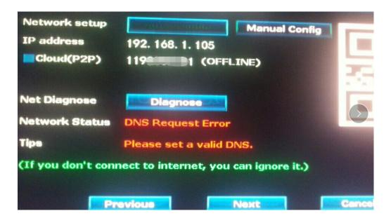
Connect the NVR to the router, right-click, select Fast network , wait for the repair to complete, can fix this error
